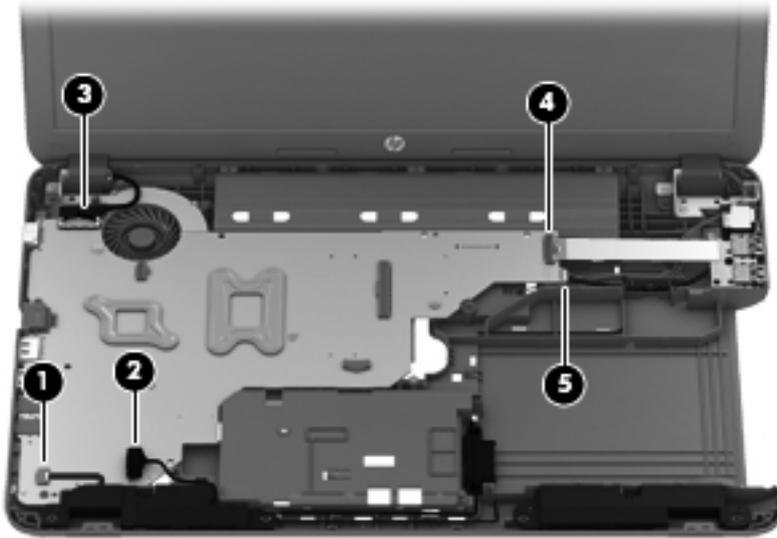
2. Remove the three Phillips PM2.5×6.0 screws **(1)** that secure the system board to the base enclosure.
