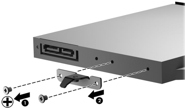
Reverse this procedure to install the optical drive.
