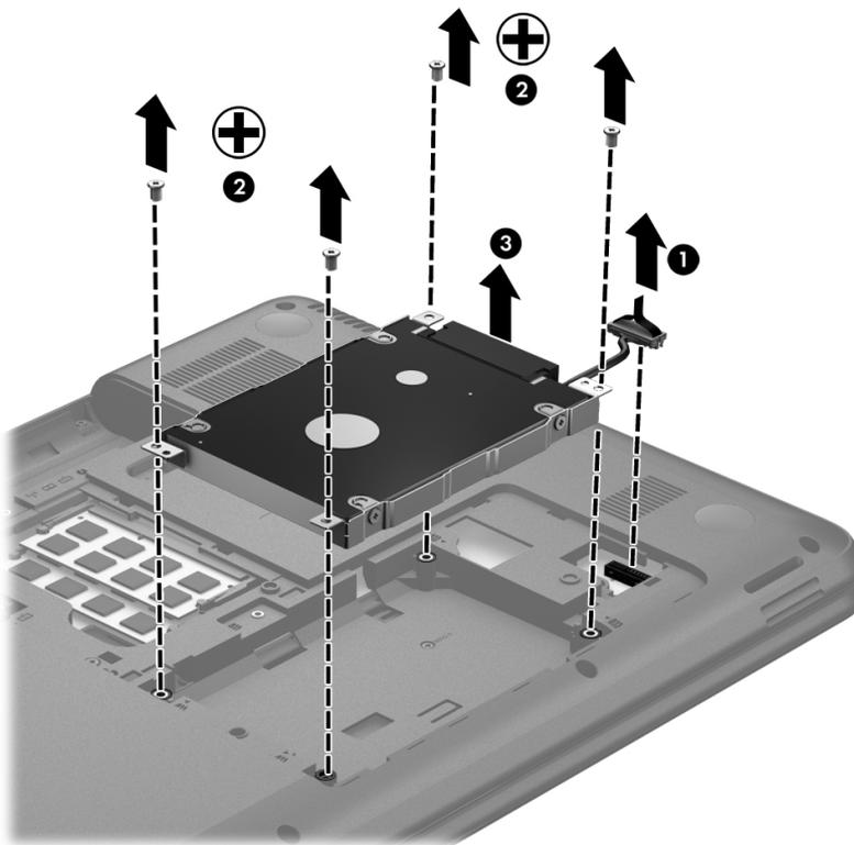
7. If it is necessary to disassemble the hard drive, perform the following steps:
