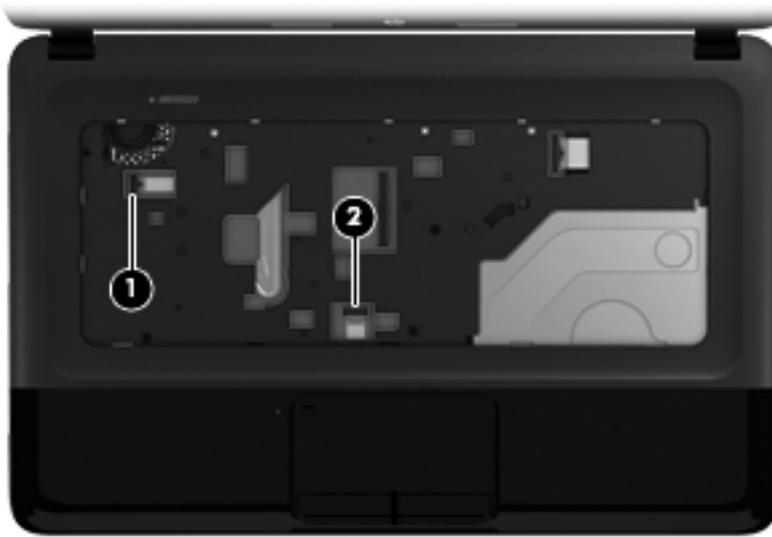
8. Remove the Phillips PM2.0×2.5 screw **(1)** and the three Phillips PM2.5×6.5 screws **(2)** that secure the top cover to the computer.
