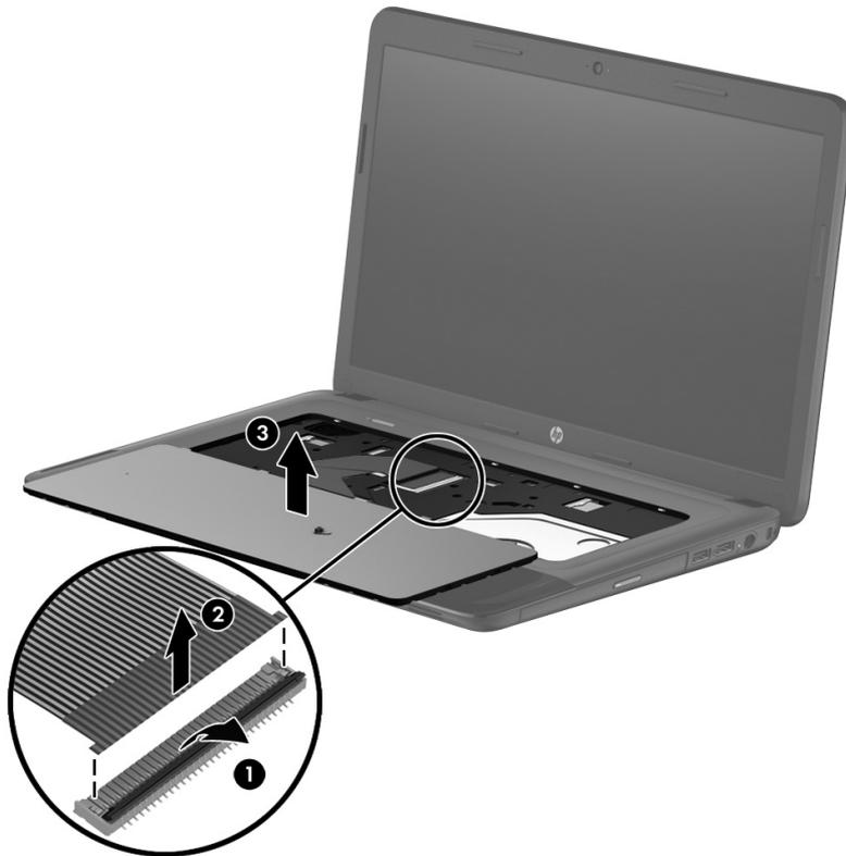
Reverse this procedure to install the keyboard.
