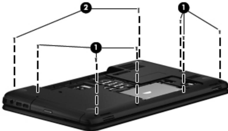
2. Remove the four Phillips PM2.0×2.5 screws on the rear edge of the battery bay and in the hard drive bay that secure the top cover to the computer.
