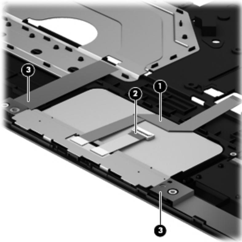
5. Remove the two Phillips PM2.5×4.0 screws **(1)** that secure the TouchPad button board to the top cover. Lift the rear edge of the TouchPad button board **(2)** until it rests at an angle.
