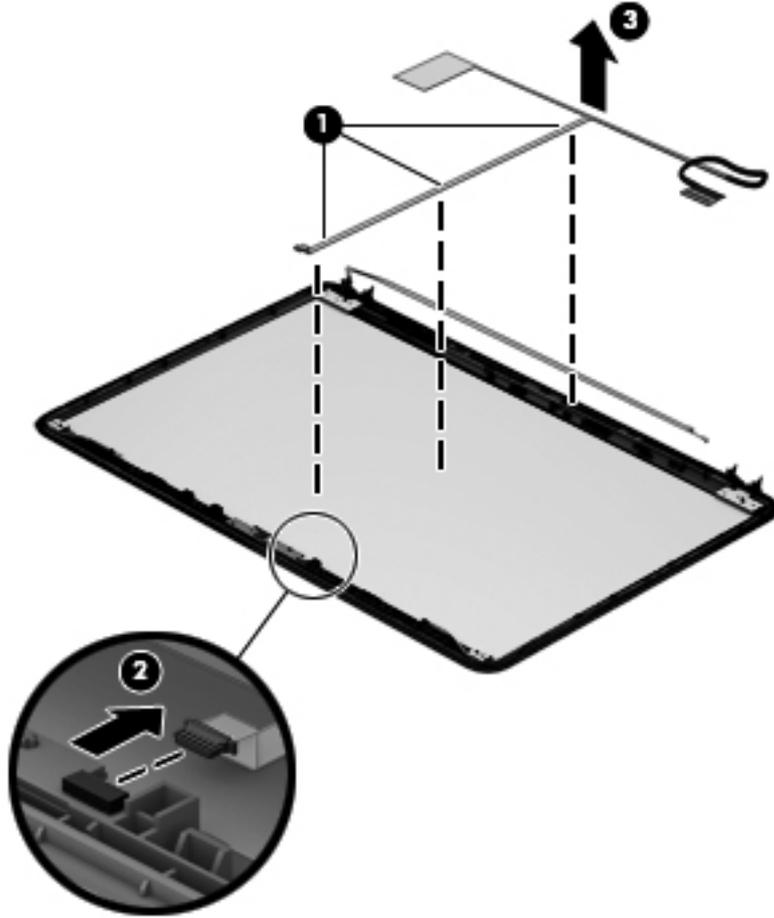
10. If it is necessary to replace the webcam/microphone module, gently detach the webcam/microphone module from the display enclosure. (The webcam/microphone module is attached to the display enclosure with double-sided tape.) The webcam/microphone module is available using spare part number 686285-001.
