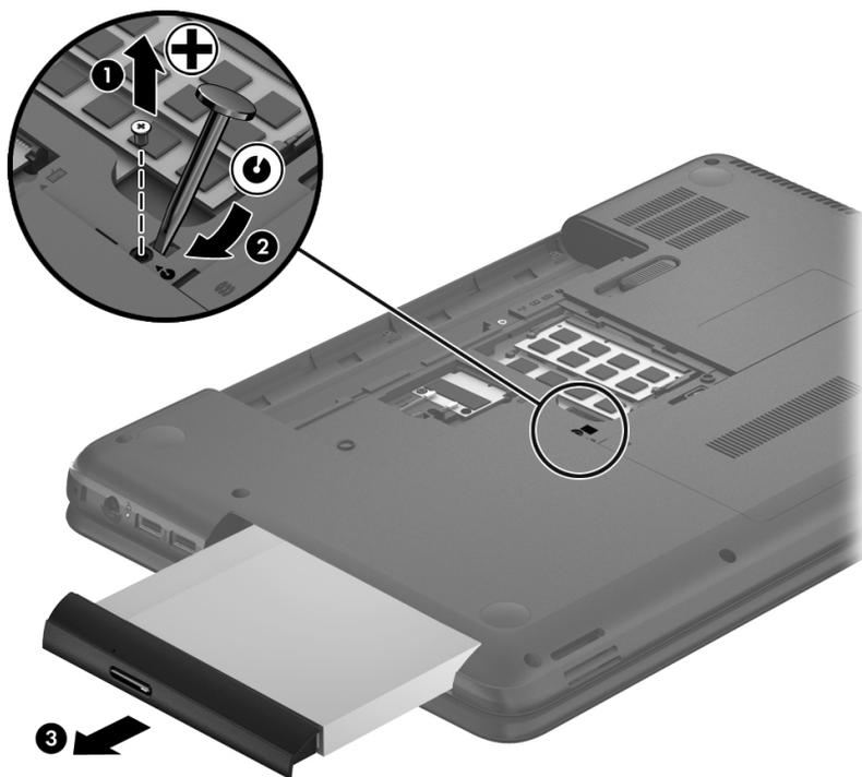
4. If it is necessary to replace the optical drive bezel, use a thin tool or an unbent paper clip **(1)** to release the optical drive tray.
